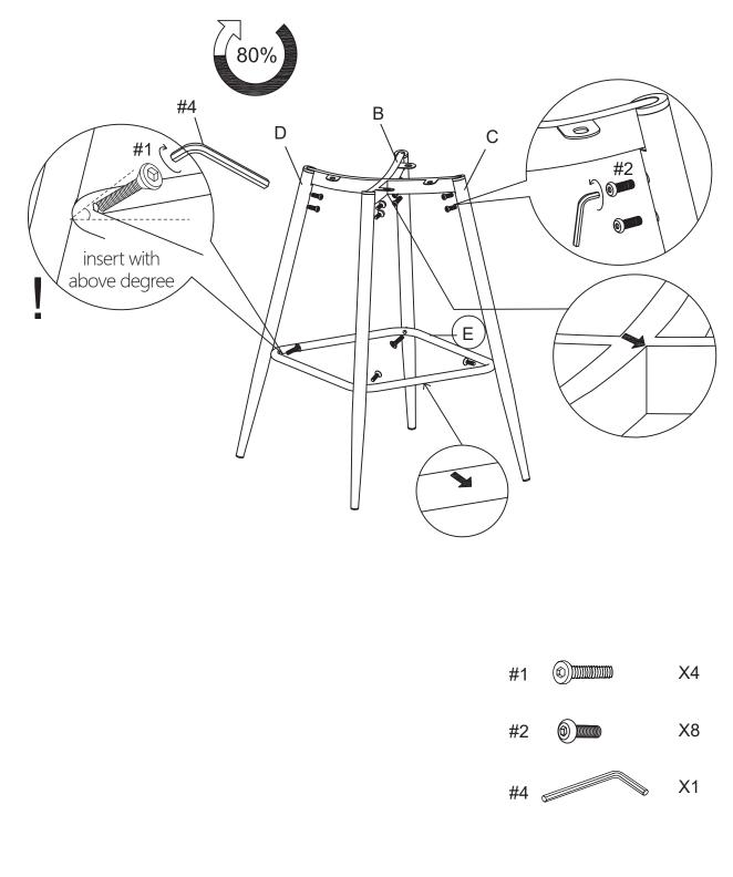
Step 3: Carefully turn seat (part A) upside down on a soft flat surface, such as carpet. Attach assembled unit (parts B, C, D & E) to seat (part A) using short bolts (part #2), flat washers (part #3) and allen wrench (part #4).
